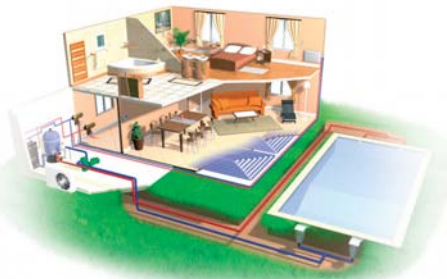
Cooling-heating floor downstairs, fan coil units or low temperature radiators upstairs, and swimming pool water heating
