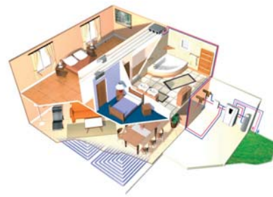
Mixed solution with heating-cooling floors downstairs and a Residenciat unit upstairs
